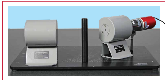
Figure 4-1: Collimated ^{137}\text{Cs} source and NaI detector positioned on the scattering table.
