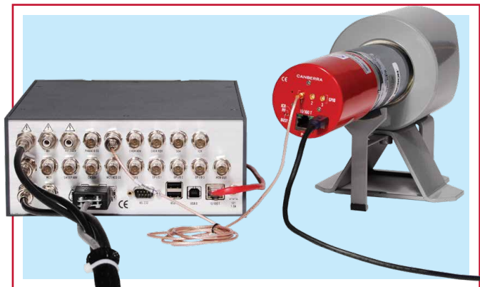
Figure 9-1: Cable configuration for synchronization of Lynx and Osprey MCAs
